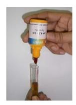
2. Add 2 drops of the Indicator. Cap the tube and invert to mix.
