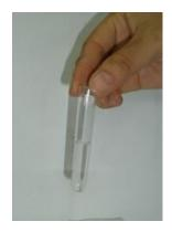
**1.** Fill the tube with 3 ml (1/2 of the tube) of sample water.
